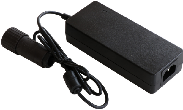
Figure 6: Power supply unit (Input: 90...240VAC, Output: 24VDC, 3.73A, 90W). See Table 3 for Pin assignment. The Pin-A and Pin-B are used only.
